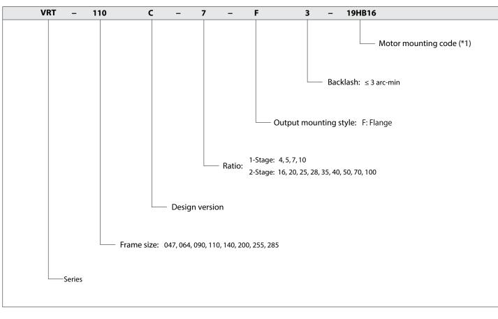
\*1) Motor mounting code varies depending on the motor. Use the selection tool link below to configure the code.
